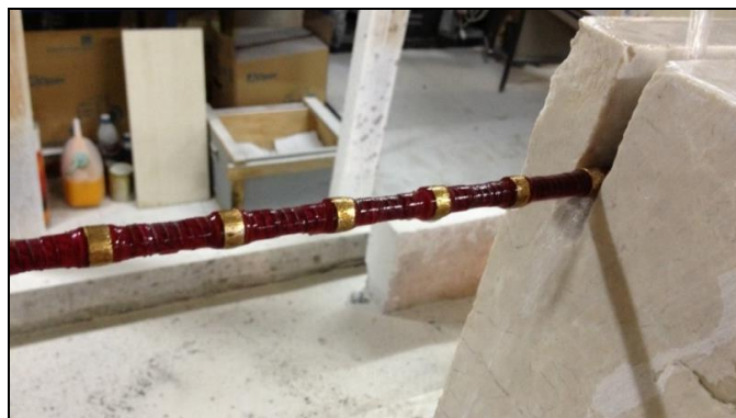
Fig. 3 Image of the diamond wire used in the experiments.
